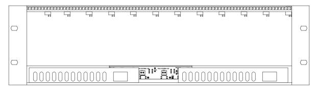
The **AMG2015-DR** is a dual redundant subrack for a standard 19" rack. It is designed to house rackmount AMG3000-5000 series video transmission equipment.
